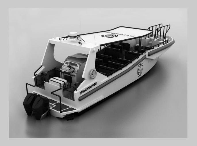
Fast Passenger boat designed as per Owner requirements for the use in Colombia waters for the transport of passengers in Santa Marta area. All passengers are protected through a height bulkwark and a bimini which protects a wide area of the passenger deck.
