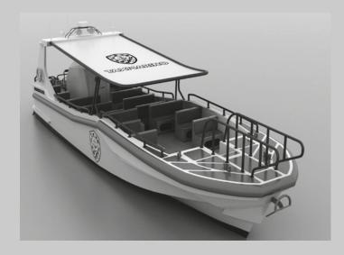
This particular boat has a length of 13.8m and a capacity of 38 passenger and 2 crew members. The maximum power to be installed is two outboard engines of 400hp each, permitting a sailing over 30kn at full load.
