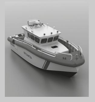
The maximum 34kn speed at full load is achieved thanks to the propulsion system equipped by two outboard MERCURY engines of 300hp each. The range of this particular boat is over the average range of this type of boats thanks to the twin fuel tanks of 600 litres each.
