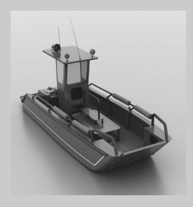
The design of this boat takes into account a possible production fabrication. For this reason, its design permits a reduction of the fabrication period and a reduction of the costs from the first constructed unit.
