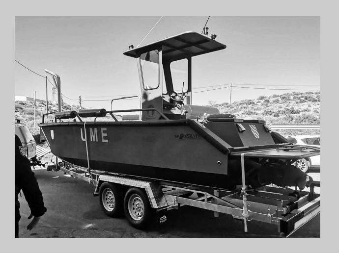
This particular boat was fully designed for "UNIDAD MILITAR DE EMERGENCIA", equipped by a forward wide landing ramp for an easy dis/embarkation besides a wide free work deck area. It's propelled by a jet and engine of 300hp making a possible 40kn sailing at full load.
